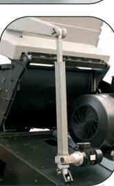
**Power-assisted** opening/closing Rapid opening and closing of the infeed hopper is assured by a motor-driven jack.
