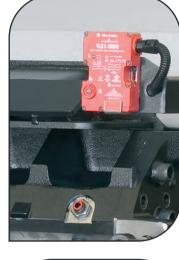
Improved safety interlock The new design of the safety interlock system allows quicker opening of a granulator. It is also safer because its speed-related sensor ensures that the rotor is standing still before the granulator can be opened.
