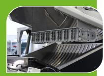
The newly designed corrugated floor opens up products it can efficiently shred.
