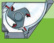
**Super-Tangential** The Super-Tangential cutterhouse is ideal for voluminous parts and scrap providing excellent grip. Standard configuration includes two fixed knives.
